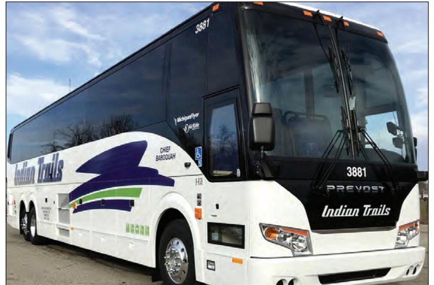
kneeling suspension to help passengers get on or off. The coaches exceed EPA standards with engine technology that cuts exhaust pollutants to near zero while achieving 240 passenger miles per gallon.
